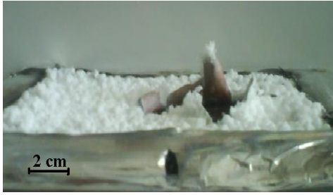
Fig. 4. Specimen after test with damaged fire protective coating side view
