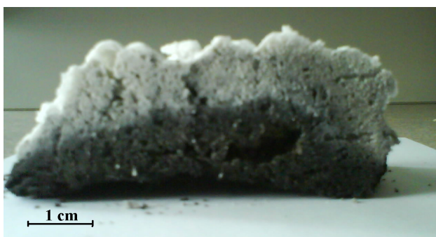
Fig. 6. Fire protective coating after exposure to high temperature: a – thickness of the formed coating h_1 is 22 mm; b – a piece of foam cut out of the specimen
